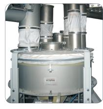
Highly precise weighing as a multi-component model.
